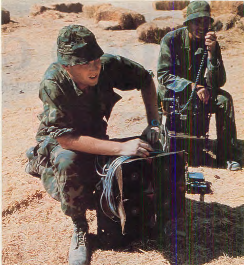
September 1969. Sailors from Beach Jumper Unit One train with 250-watt, man-portable loudspeaker and portable telephone of type used in Vietnam. Photo: DoD
